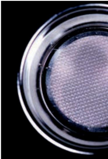
IMS has created an innovative and unique product for finer filtering even using an espresso machine. The level of filtering is normally between 250  $\mu\text{m}$  and 350  $\mu\text{m}$ . The Super Fine filter has a level of filtering of 170  $\mu\text{m}$ . To achieve this IMS combined the benefits of a photo-etched membrane with its own perforation technology. This results in a cleaner espresso that accentuates the acid component of coffee.
